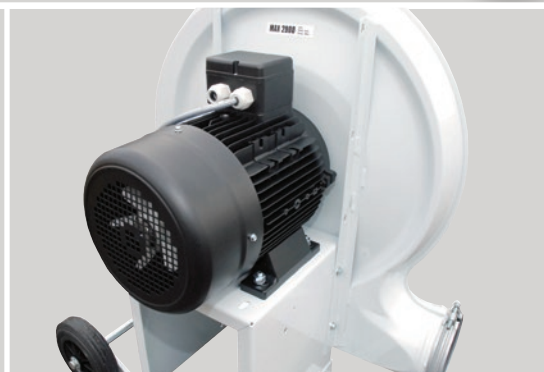
The motor directly drives the blower rotor
